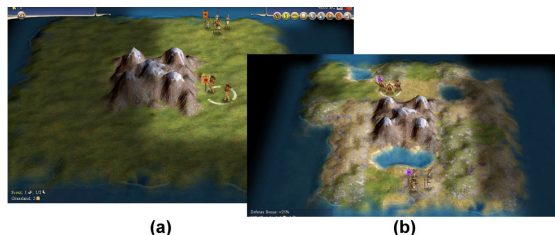
Figure 4. An application of Harp where the generative information is based solely on the position of the pattern in the automaton generates several identical islands (a). When each pattern is affected by nearby patterns, more detailed and differentiated landmasses are generated, such as the one depicted in (b).
