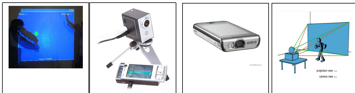
Figure 1: The figures above illustrate: the game Shadow Volleyball (first figure, left), the use of a “pocket projector” connected to a mobile phone, the Samsung W7900 mobile projector phone and the projector and camera setup used during the tests.
